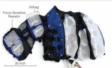
Figure 3. Force Jacket with internal airbags layout exposed.
